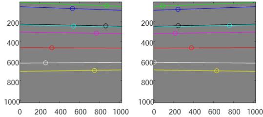
Figure 3: A set of matching points and the corresponding epipolar lines, that were simulated using the parameters of the example in Fig.2.
