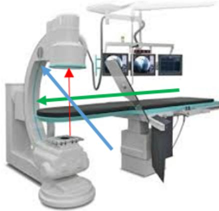
Figure 1: An angio system. The ISO center is located at the coordinates' origin. The plotted axes are the axes along which the bed may be translated and around which the C-arm may be rotated
