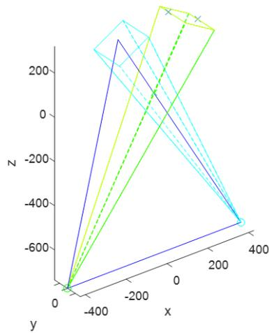
Figure 2: Simulation of two possible states of the angio system. The head of each pyramid is the x-ray source and the pyramids' bases are the detectors location. The intersection area of both pyramids includes the location of the patient's heart, in case the bed translation was equal in both positions. In this example, the C-arm was rotated once towards the left side of the patient and once towards the right, and was not rotated around the other axes. The blue triangle marks an epipolar plane.
